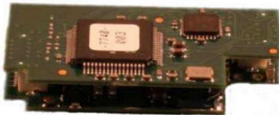
(TS//SI//REL) FLUXBABBITT Hardware Implant for PowerEdge 2950
