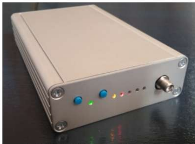
(U//FOUO) HackRF One with optional enclosure
